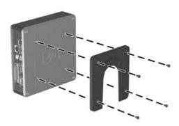
Figure 5-2 Connecting the HP Quick Release to the thin client
